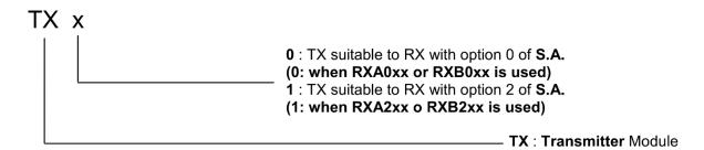
The codes identifying AL module of DSP LASER with the corresponding configuration are:
