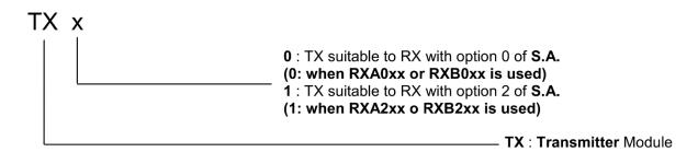
The codes identifying AL module of DSP LASER with the corresponding configuration are:
