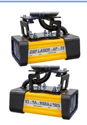
DSP AP emits a **visible laser barrier** which, made and placed as described in the EN12622 standard, **protects the press brake operator** against the risk of being crushed between the upper and lower part during the closing of the fold at high speed.
