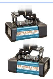
DSP emits a **visible laser barrier** which, made and placed as described in the EN12622 standard, **protects the press brake operator** against the risk of being crushed between the upper and lower part during the closing of the fold in high speed.
