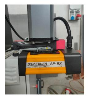
Therefore, align the B-Sniper 02 device so that the laser trace is projected to the center of the matrix and align the DSP Laser photocell last.
