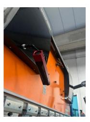
Equipped with rechargeable batteries and a battery charger, the B-Sniper 04 with its **articulated magnetic arm** is **very easy to attach** to the press brake and is **immediately ready** for use.
