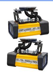
DSP AP emits a visible laser barrier which, made and placed as described in the EN12622 standard, protects the press brake operator against the risk of being crushed between the upper and lower part during the closing of the fold at high speed.
