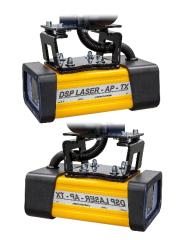
DSP AP is a visible laser emission barrier which, realized and placed as described in Standard EN12622, protects the operator of the press brake against the danger to be squashed between the upper and the lower tool during the closing of the press in high speed.
